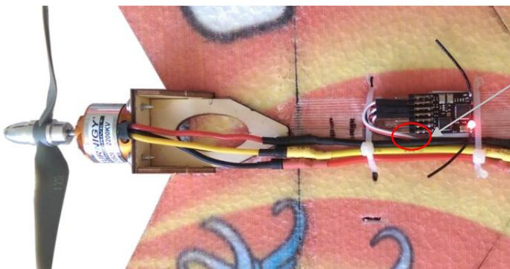
Servo wires from the V-tail mixer below exit here and plug into the elevator and aileron servo ports on the receiver.
