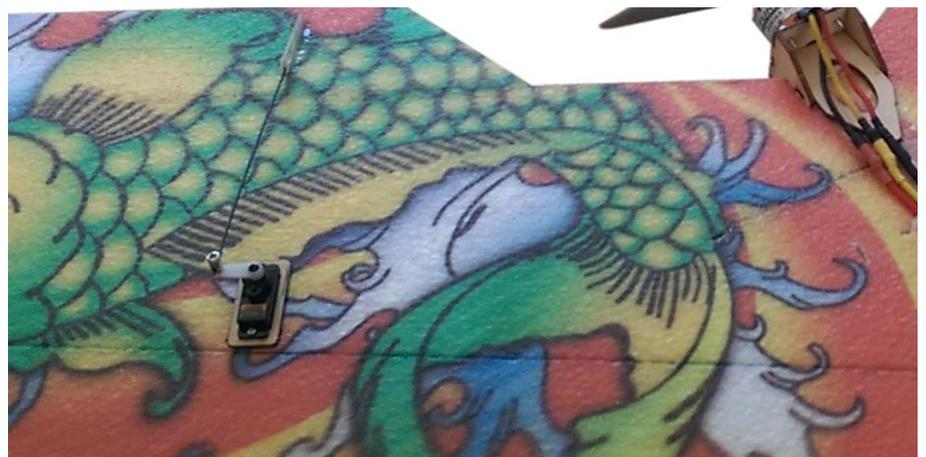
Note: Lay out your servos on the wing and connect up your receiver and v-tail mixer before starting the fitout. Check that servo arms are moving in the correct direction or that you are able to adjust your transmitter servo reversing if required.
